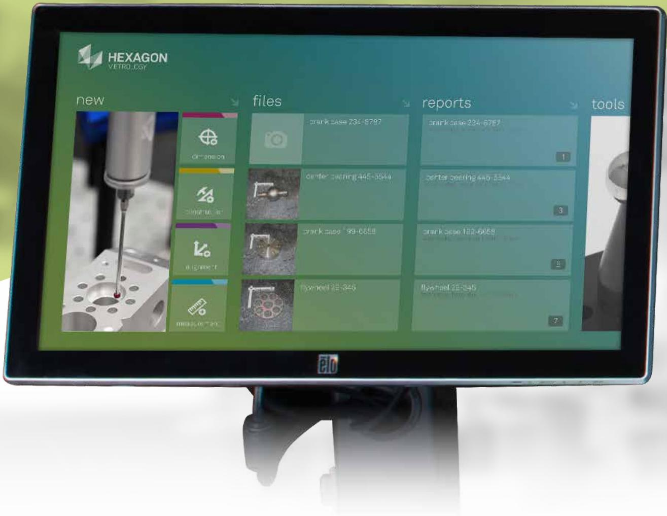
The SF series includes PC-DMIS®, today's most popular and powerful metrology software, featuring an intuitive graphical user interface that easily guides first-time operators through part programming, setup and inspection. It is ideal for the shop floor:
